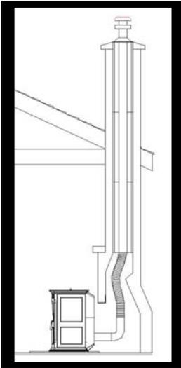
A full liner is used to reline the chimney. The liner generally allows the flue to be easily cleaned.
