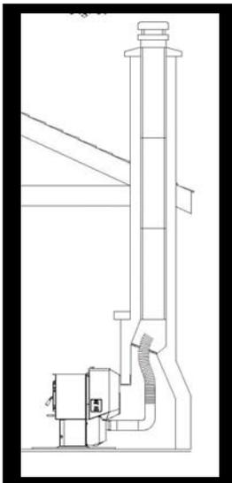
Stove is installed in front of a masonry fireplace. Vent pipe extends above the damper to just below the tile liner of the chimney.
