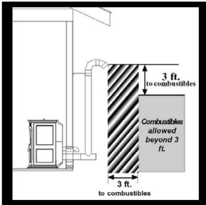
Note that the tee on the outside is positioned so that the horizontal section of the pipe can be cleaned by removing a cap on the end of the tee. An outside air kit is shown.
