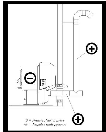
◆ Never use B Vent or aluminum dryer pipe or mix and match brands of pellet pipe to vent your stove. Aluminum pipe will melt at high temperatures. The inner liner of pellet vent pipe (PL vent) is stainless steel for this reason.
