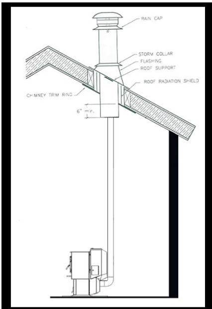
In this installation PL vent pipe is used as a connector pipe between the stove and a Class A All Fuels chimney.
