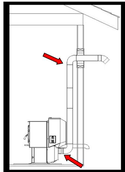
◆ The longer the vent pipe and more elbows used in the system the greater the flow resistance. We recommend as few elbows as possible (2 or 3 are OK, but 4 may be too many depending on the length of pipe between elbows) and 15 ft or less of vent pipe. 45° elbows are better than 90° elbows. The maximum horizontal run should not exceed 48”. If elbows and longer runs are unavoidable upsize to 4” PL Vent.
