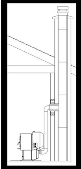
PL vent is used as a connector pipe between the stove and the masonry chimney.
